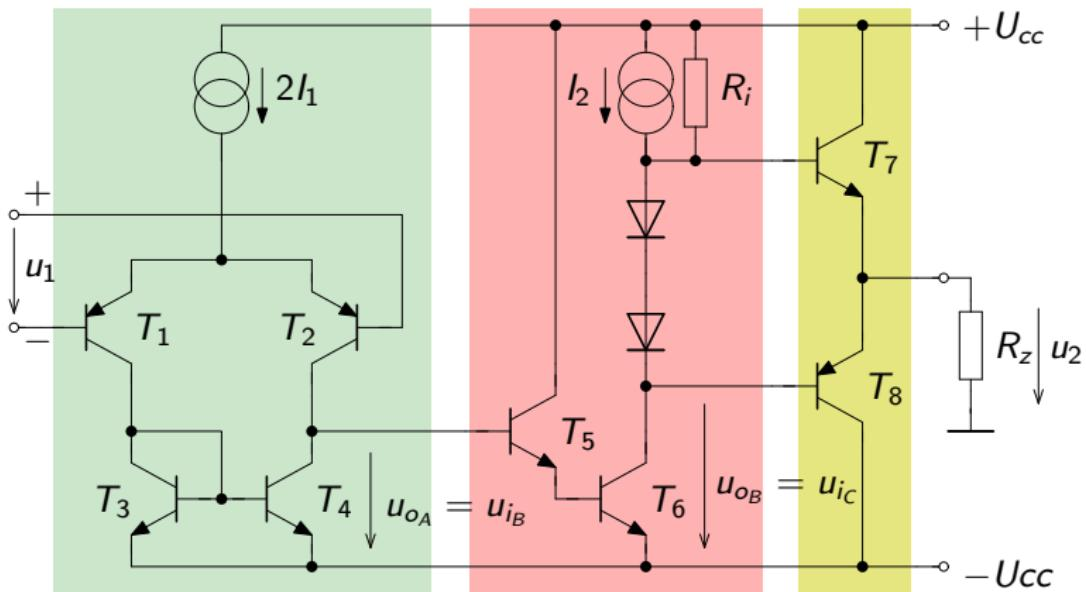
$$A_{uA} = \frac{u_{oA}}{u_1} = -g_m(r_{oA} || r_{iB}) \doteq -280, A_{uB} = \frac{u_{oB}}{u_{iB}} = -\frac{g_{m6}(r_{oB} || r_{iC})}{2} \doteq -890,$$
