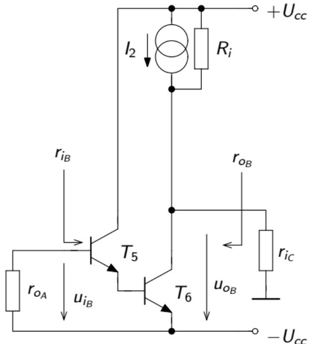
$$r_{iB} = (\beta + 1)(r_{e5} + r_{\pi6}) = \\ = (\beta + 1)2r_{\pi6} = 2r_{\pi5}$$
