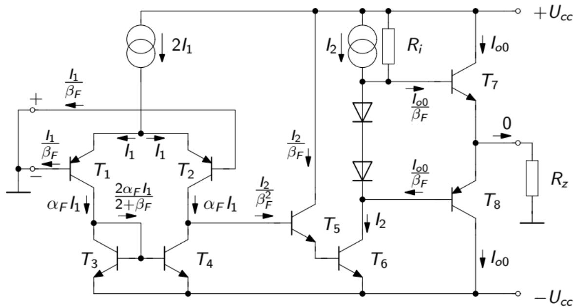
$$I_{in} = 80 \text{ nA}, I_{out_{max}} = 20 \text{ mA}, \beta_F = \beta = 80, U_A = 100 \text{ V}, R_z = 2 \text{ k}\Omega$$
